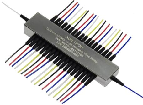
The MEMS Series N-bit (up to 18-bit) Photonic Time Delay digitally varies the delay time inside a fiber with exceptionally large range (maximum delay) and precision (bit). It selectively routes optical signals through N fiber loops whose lengths increase successively by a power of 2. Since each switching element allows the signal to either pass or bypass a fiber loop, a delay T may be inserted, which can take any value (in increments of  $\Delta T$ ) up to the maximum value T.
